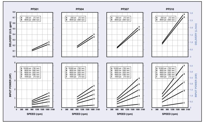
Typical performance curves are based on 100 SUS (20 cSt) mineral oil with pressurized inlet where required. Refer to the "Minimum Inlet Pressure" table on page 2. Contact the Dynex sales department for applications requiring continuous duty operation at speeds higher or lower than shown.
